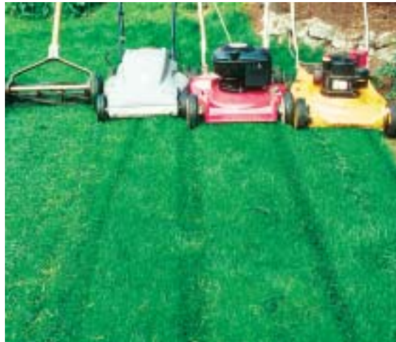
You can grasscycle with any mower. Push mowers (left) and conventional power mowers (right) leave clippings on the surface to break down. Electric and gas mulching mowers (center) blow chopped clippings down to the soil, leaving a clean lawn.
